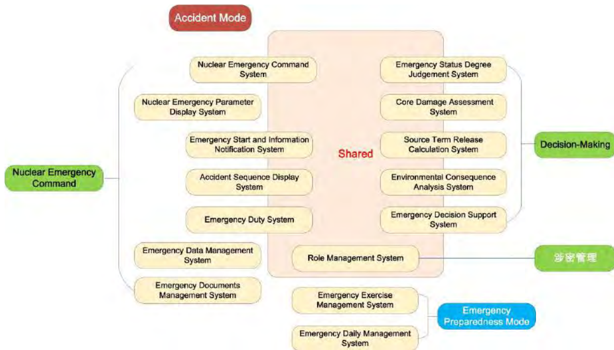
Figure 2: Main systems included in the Integrated Nuclear Emergency Command and Decision Support System for Nuclear Power Plant
