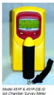
Figure 10: The ion survey meter employed to conduct the shielding test: Detection specifications Beta >1 MeV Gamma >25 KeV
