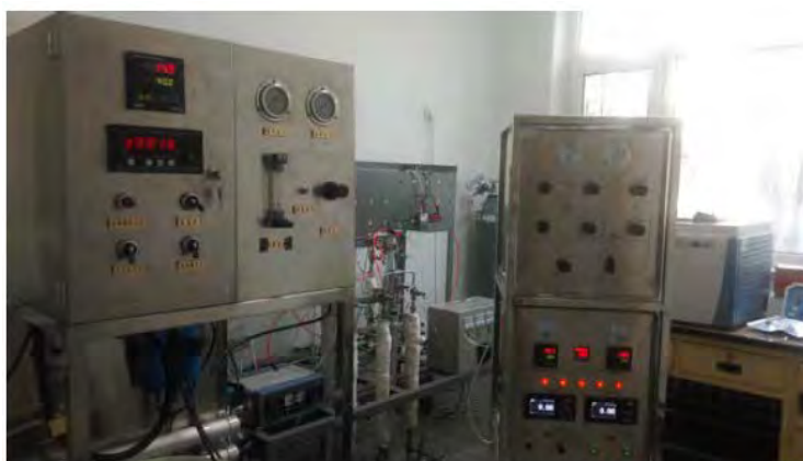
Figure 5: The prototype device of sampling and measuring the Kr-85 in the atmosphere
