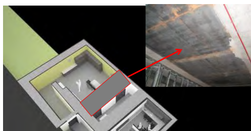
Figure 8: 17500kg steel shielding section
