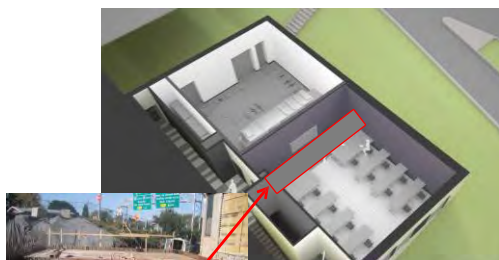
Figure 9: 17500kg steel shielding section
